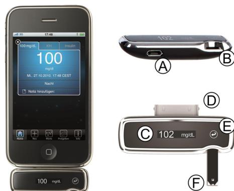
**Fig. 1:** Blood glucose meter iBG-Star; A: Micro USB Connector; B: Slot to insert testing strip; C: Liquid Crystal Display; D: 30 pin connector for Apple devices; E: Interaction button for standalone use; F: Inserted blood glucose testing strip
